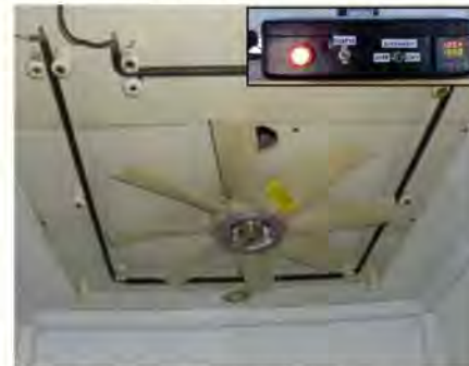
The fan and heater are installed on the ceiling of the cabinet. A PID controller (inset) rests on top of the cabinet and ensures temperature control.
