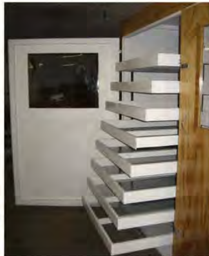
Different hop varieties can be kept separate in the oast by placing them in different trays. A total of 8 trays can be accommodated in each cabinet. Wire mesh is used as the bottom for the trays which allows air flow through the hops.
