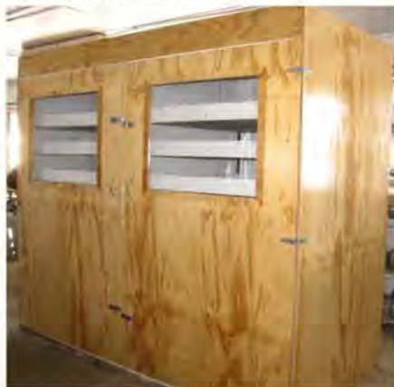
The oast includes two 4'x4'x8' cabinets with independent access doors and controls. Total capacity is 600 lbs wet hops which can be dried in 8 hours.
